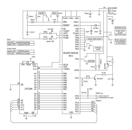
Note: This circuit is recommended for programming only at 25°C and not for use in the end application, or at temperatures other than 25°C. If used in the end application, VPP6 should be tied to VDD to avoid damaging the device.
