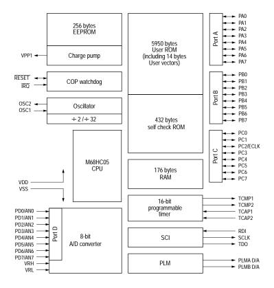
Figure 1-1 MC68HC05B6 block diagram
