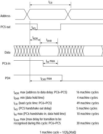
Figure C-10 RAM parallel loader timing diagram
