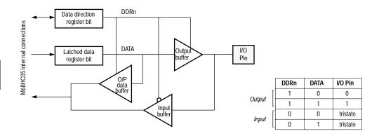
Figure 4-1 Standard I/O port structure
