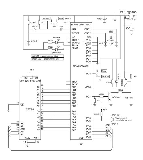
Note: This circuit is recommended for programming only at 25°C and not for use in the end application, or at temperatures other than 25°C. If used in the end application, VPP6 should be tied to VDD to avoid damaging the device.
