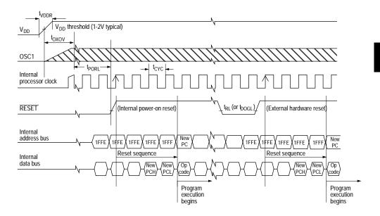
Figure 9-1 Reset timing diagram
