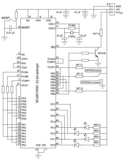
Note: For the MC68HC05B4, switches on PB5 and PB6 have no effect All resistors are 10 kΩ, unless otherwise stated.
