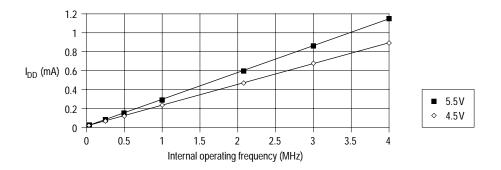
**Figure 11-2** Run  $I_{DD}$  (SM = 1) vs internal operating frequency (4.5 V, 5.5 V)
