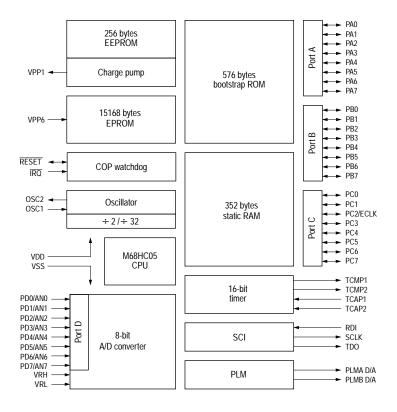
Figure F-1 MC68HC705B16N block diagram
