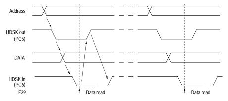
Figure C-5 Timing diagram with handshake
