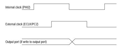
Figure 4-2 ECLK timing diagram
