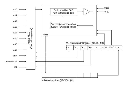
Figure 8-1 A/D converter block diagram
