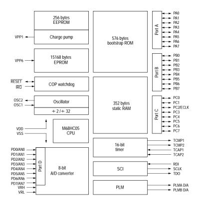
Figure E-1 MC68HC705B16 block diagram
