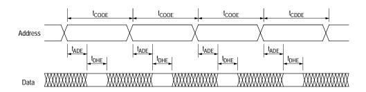
$t_{ADE}$  max (address to data delay) 5 machine cycles  $t_{DHA}$  min (data hold time) 14 machine cycles
