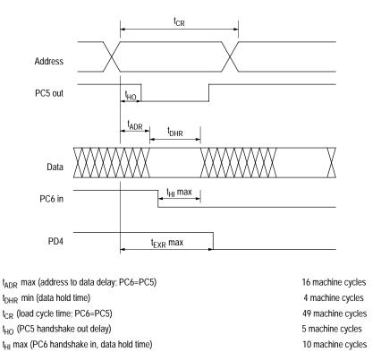
Figure H-9 Parallel RAM loader timing diagram
