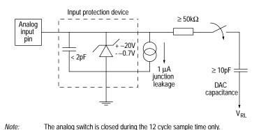
Figure 8-2 Electrical model of an A/D input pin
