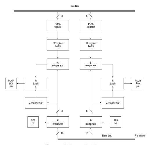
Figure 7-1 PLM system block diagram
