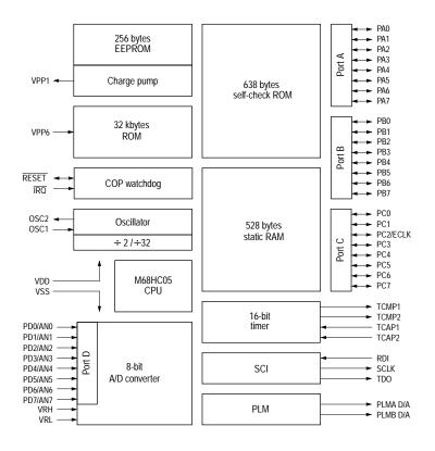
Figure G-1 MC68HC05B32 block diagram
