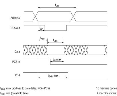
Figure F-9 Parallel RAM loader timing diagram
