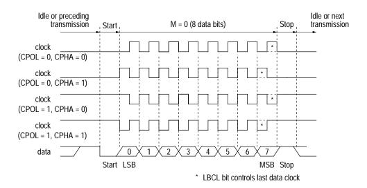
Figure 6-9 SCI data clock timing diagram (M=0)
