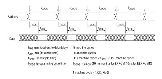
Figure F-6 Parallel EPROM loader timing diagram
