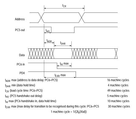
Figure E-9 Parallel RAM loader timing diagram
