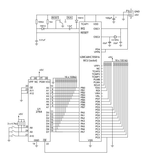
Figure E-10 RAM parallel bootstrap schematic diagram
