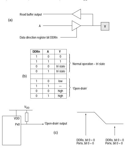
Figure 4-3 Port logic levels
