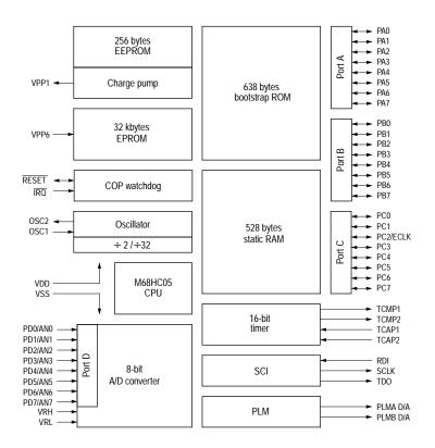
Figure H-1 MC68HC705B32 block diagram
