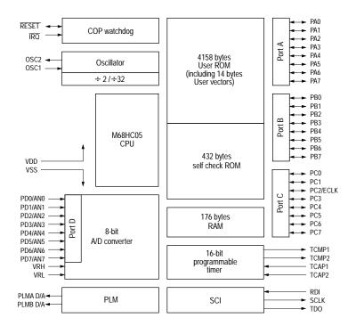
Figure A-1 MC68HC05B4 block diagram
