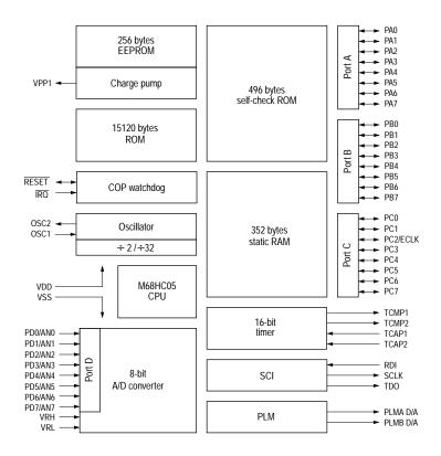
Figure D-1 MC68HC05B16 block diagram
