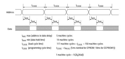
Figure H-6 Parallel EPROM loader timing diagram
