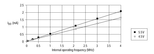
Figure 11-3 Wait I<sub>DD</sub> vs internal operating frequency (4.5 V, 5.5 V)
