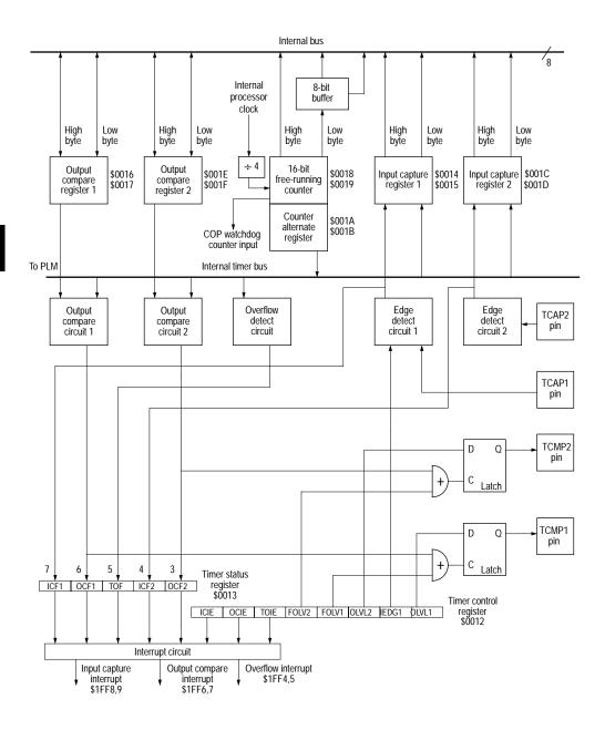
Figure 5-1 16-bit programmable timer block diagram
