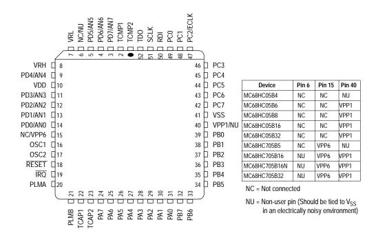
Figure 12-1 52-pin PLCC pinout for the MC68HC05B6
