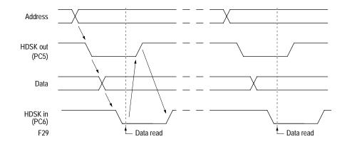
Figure F-5 Timing diagram with handshake
