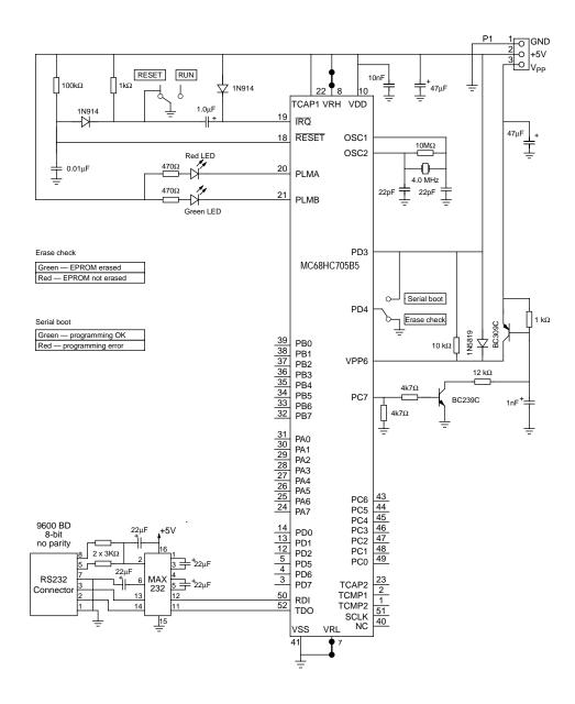
Note: A minimum V<sub>DD</sub> voltage must be applied to the VPP6 pin at all times, including power-on, as a lower voltage could damage the device. Unless otherwise stated, EPROM programming is guaranteed at ambient (25°C) temperature only
