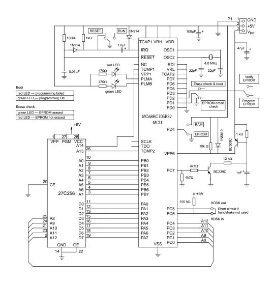
This circuit is recommended for programming only at 25°C and not for use in the end application, or at temperatures other than 25°C. If used in the end application, VPP6 should be tied to VDD to avoid damaging the device.
