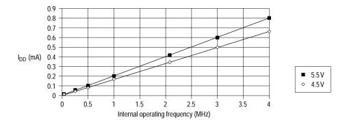
Figure 11-4 Wait I<sub>DD</sub> (SM = 1) vs internal operating frequency (4.5 V, 5.5 V)
