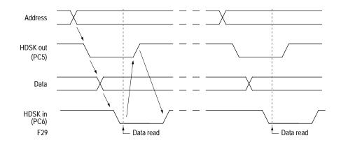
Figure H-5 Timing diagram with handshake
