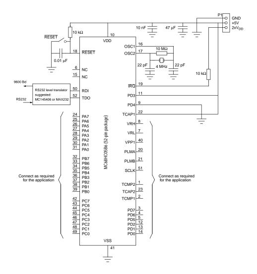
Figure 2-1 MC68HC05B6 'load program in RAM and execute' schematic diagram
