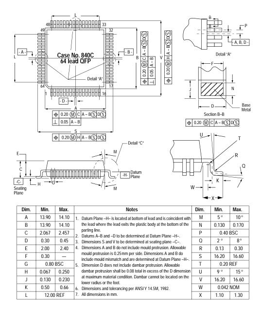
Figure 12-5 64-pin QFP mechanical dimensions
