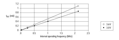
Figure 11-9 Wait I<sub>DD</sub> vs internal operating frequency (3V, 3.6V)
