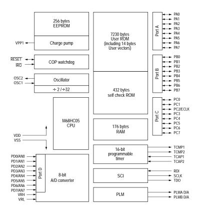
Figure B-1 MC68HC05B8 block diagram
