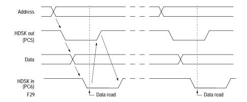
Figure E-5 Timing diagram with handshake
