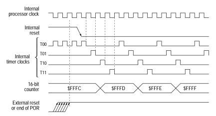
Note: The counter and timer control registers are the only ones affected by power-on or external reset.
