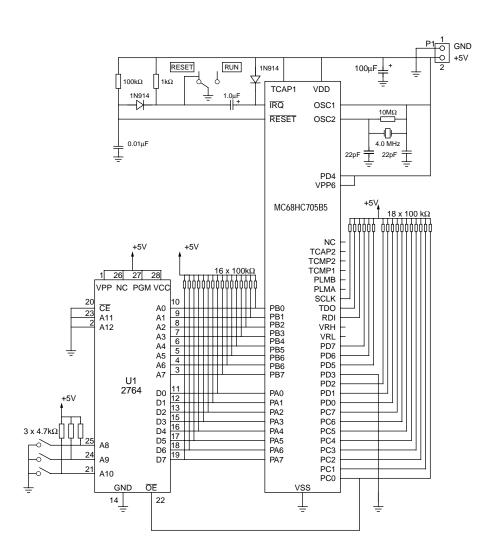
Figure C-8 RAM parallel bootstrap schematic diagram
