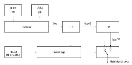
Figure 2-4 Slow mode divider block diagram
