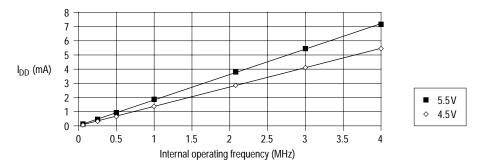
Figure 11-1 Run I<sub>DD</sub> vs internal operating frequency (4.5 V, 5.5 V)
