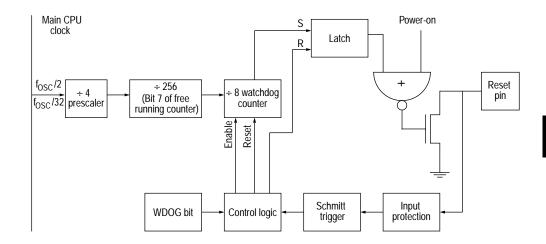
Figure 9-2 Watchdog system block diagram
